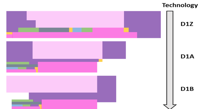
Fig. 2. Layout changes in a IP with the same schematic. Different color represents the floorplan area for different type of components*.
